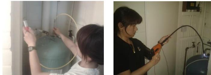
**Figure 3-7 (Left) Meg Uapipatanakul from the Oxford Microbiology Research Group taking samples from bottom of tank using sample probe (right) endoscope camera inserted to take images of bottom of tank**
