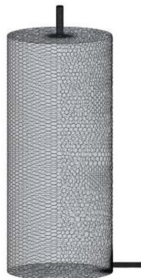
**Figure 5-12 Mesh applied to empty tank**
