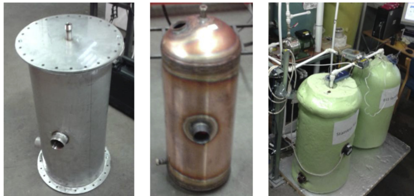
Fig. 3. (Left) Stainless steel tank, (center) copper tank, (right) insulated tanks under test.
